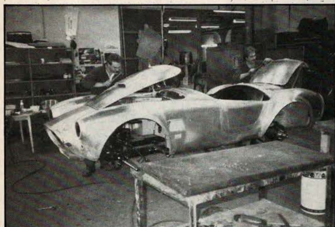
Although the layman may not see it, there are imperfections in the body and these two Gents are responsible for making sure the aluminum body is smooth as, ahem, glass. And we don't mean fiberglass.
