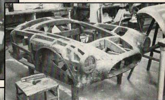
This wood buck, or form, is also an AC original. The years of use have left it none the worse for wear.
